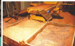
Cables are separated into their constituent elements.
