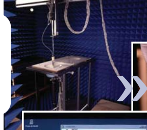
Dosimetry: a SAR test bench in an anechoic room
