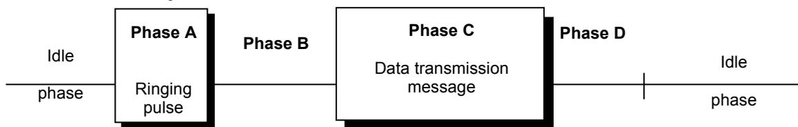
Figure 3: The various phases involved in the data transmission procedure
